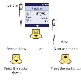
In Pip and Dis mode, press the rocker in the opposite direction of the piston movement to stop it. Afterwards, press the rocker up or down to move the piston in the desired direction.
